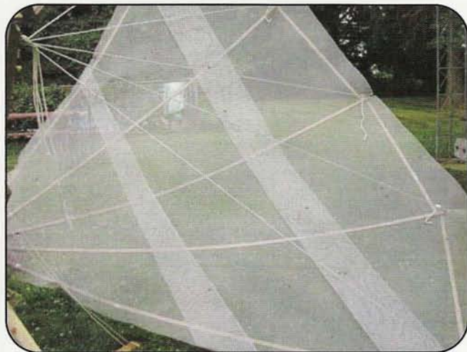
Photo H. Aluminum screening is tied to the struts using wire.
