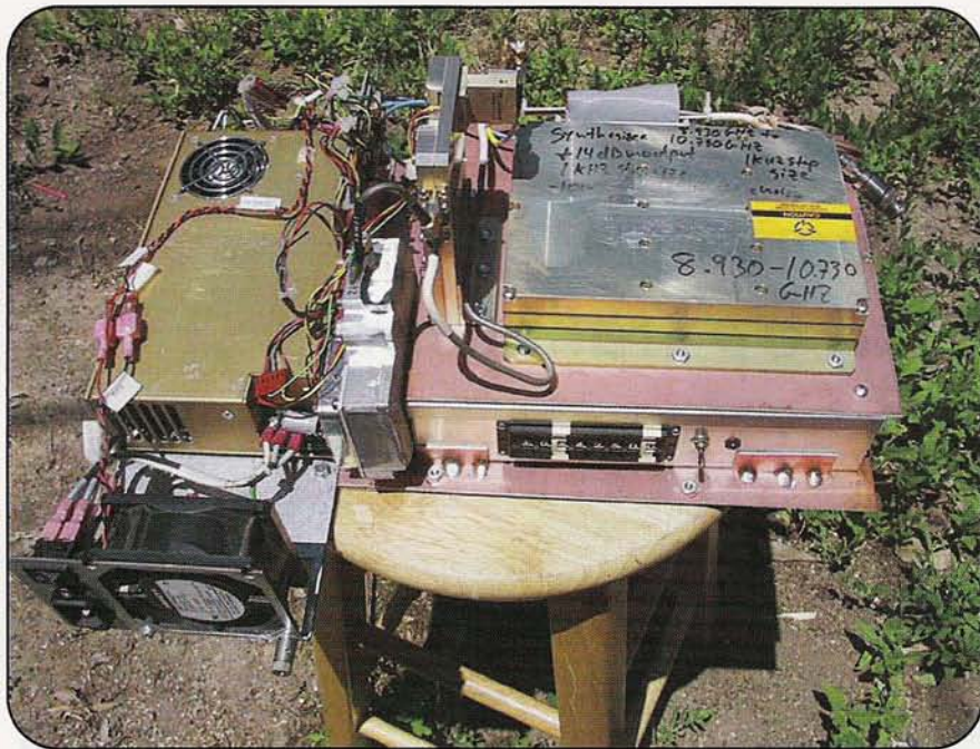
Photo B. Top view of the 47-GHz rig. The Verticom synthesizer is to the right. The 2640-MHz synthesizer is at the bottom left in the aluminum cutout shield compartment. The Pecom 23-GHz TX module is just above the 2640-MHz synthesizer. The switching regulated power supply is to the far left, with the cooling fan in front of the power supply.
