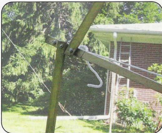
Photo C. An outside rim is formed from 3.5-foot length of 1/2" \times 1/2" modeling strips.
