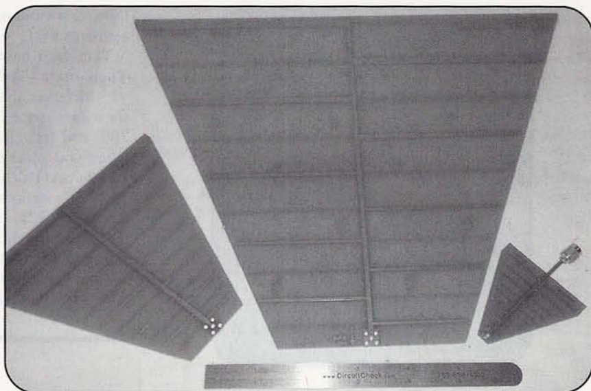
Photo H. PC-board log-periodic antennas from 400 MHz to 11 GHz.
