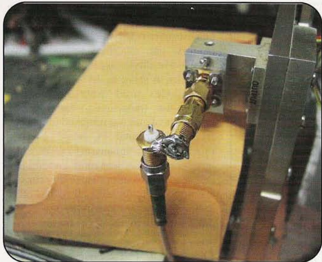
Photo C. Close-up of the 47-GHz system mixer showing the tiny diodes (you can barely see them) and IF cable (145 MHz) and SMA connector pointing downward in the original test configuration. This was the first design.
