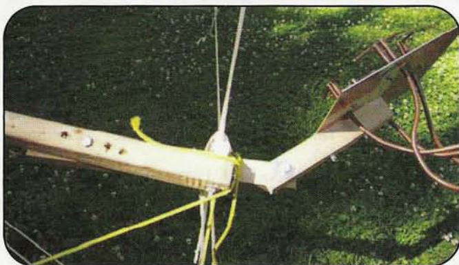
Photo E. The feed is mounted using several supports to allow optimum positioning.
