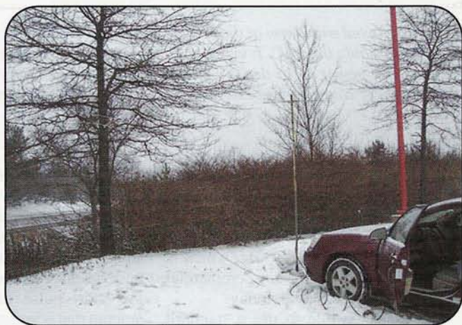
Here is WB2AMU's QRP setup on one of the hills on Long Island at the beginning of the January 2005 VHF Sweepstakes just before the blizzard began. The 2-meter beam is in the umbrella stand in front of the car, and the two-element, 6-meter beam is in the tree to the left. After 45 minutes the action cooled down, and it seemed like a good time to cease operation, given that over 15 inches of snow would fall overnight. (Photos by Ken Neubeck, WB2AMU)
