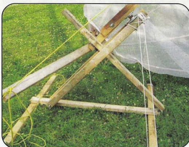
Photo F. The base of the polar mount is made from six 4-foot lengths of 2" \times 3" lumber.
