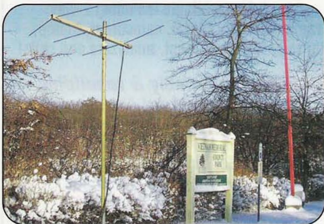
Here the three-element, 2-meter Yagi is facing west from Bald Hill on Long Island (grid FN30) just moments prior to WB2AMU working W2FU (grid FN13) on CW in western New York via an apparent tropo-ducting enhancement on 2 meters.
