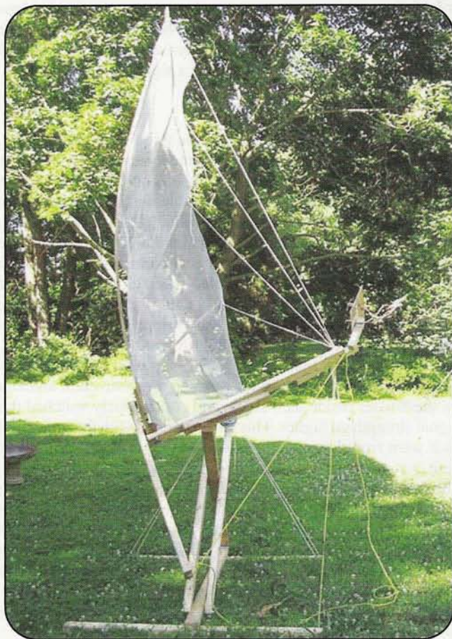
Photo A. A 7.5-foot offset dish on polar mount. (All photos courtesy of the author)
