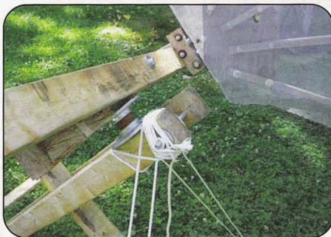
Photo G. A 1-inch diameter pipe nipple is used for the polar axis.
