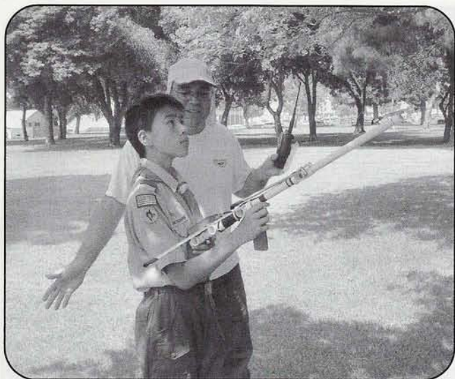
Is it in the tree? This Scout is using my 2-meter on-foot RDF set, which has a handle at the exact balance point to avoid wrist fatigue. Helping him is Tom Gaccione, WB2LRH. (Photo by KØOV)
