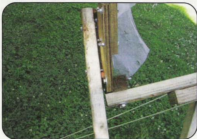
Photo D. The dish is attached to the feed support by a 2" \times 2" block.
